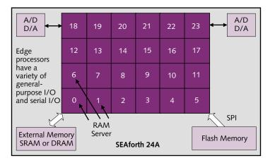
**Figure 1.** Both of the first two SEAforth chips have an array of 24 processor cores. All the 18-bit processor cores are functionally identical, but some perform different tasks. In particular, cores at the edges of the chip handle various I/O duties.
