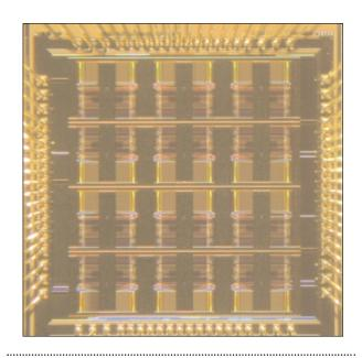
**Figure 3.** The SEAforth-24A embedded array integrates 24 identical processor cores with on-board serial and parallel I/O ports plus A/D and D/A converters.
