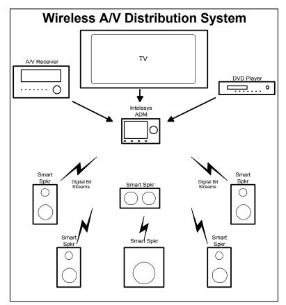
then, the mesh network would consist of seven nodes, one at the A/V receiver and six at the speakers. All would be symmetric in the sense that they share most or all of the same hardware. Likewise the speaker nodes would be identical in that they all share exactly the same computer code. While all speakers would receive the entire bit stream, each speaker would simply extract the audio information for that specific speaker.
