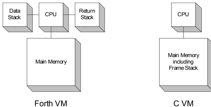
By adding the necessary registers for the frame stack to the canonical Forth machine, we arrive at the basic design of the SENDIT VM, which was discussed in various papers in the late 1990s. SENDIT (EP9152) was a project carried out under the European Union's ESPRIT research and development programme. SENDIT was based upon the results of a preceding project, PROCIC EP5497, and produced tools for the development of heterogeneous networks for use in embedded and real time applications.
