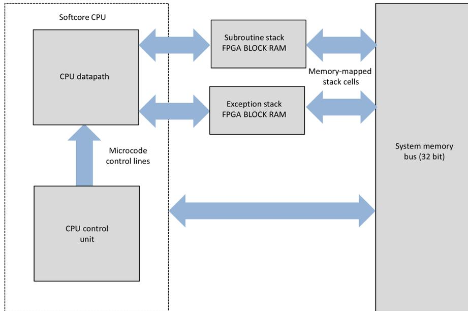
Figure 9: System diagram of the extended return stack implementation on the N.I.G.E. Machine
