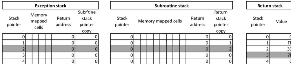
Figure 7: Application of the extended return stack model to FORTH with an exception, subroutine and return stack. The additional memory-mapped cells on the subroutine and exception stacks are shown narrower for clarity of the diagram only.
