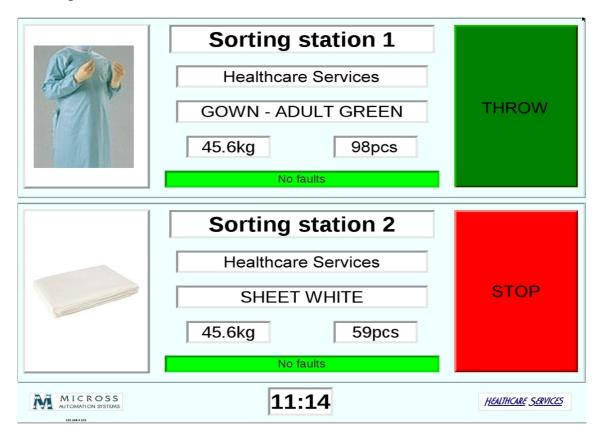
In the example shown on the previous page, the display unit shows the status of two healthcare laundry sorting stations. The customer, category, weight and piece count are shown. The category is illustrated for quick identification. Indicator beacons show the operator clearly when to sort items. This application was implemented using Python.
