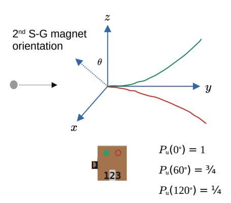
Simulation output from epr-sim for 0°, 60°, and 120°.
